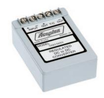
Input/output isolation prevents ground loops, and permits the use of inputs of either polarity; outputs of single output models may be used in either polarity and floated up to 500 volts above the input. Short circuit and thermal protection, and rugged encapsulated construction, assure years of reliable service.
