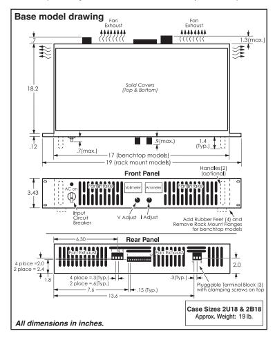
**Mounting:** Rack Mounting models are designed expressly for mounting in standard 19" wide RETMA cabinet racks. Benchtop models rest on four rubber feet.
