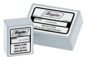
Efficiency is in the order of 65%, and is maintained down to low levels of output current. Input reflected ripple is reduced to less than 1% by means of a standard built-in pi filter, and electrostatic shielding on all six sides minimizes radiated energy. High input/output isolation permits separation of the output from the dc input bus to minimize circuit interaction due to ground loops, and the use of inputs in either polarity.
