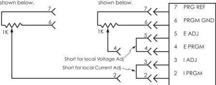
Do not remove jumper between pins 2 and 3 if remote current adjustment is not used, or between pins 4 and 5 if remote voltage adjustment is not used.
