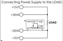
THE DOTTED LINE CONNECTION IS REQUIRED. unless remote voltage adjustment is used. A potentiometer OR switched resistors in the negative sense lead may be used to remotely program (adjust) the output voltage:
